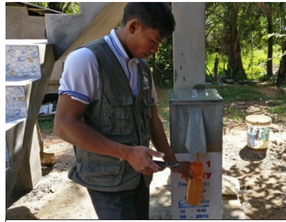
WFC staff member Hun samples filter output from a recent installation for lab analysis to ensure proper
